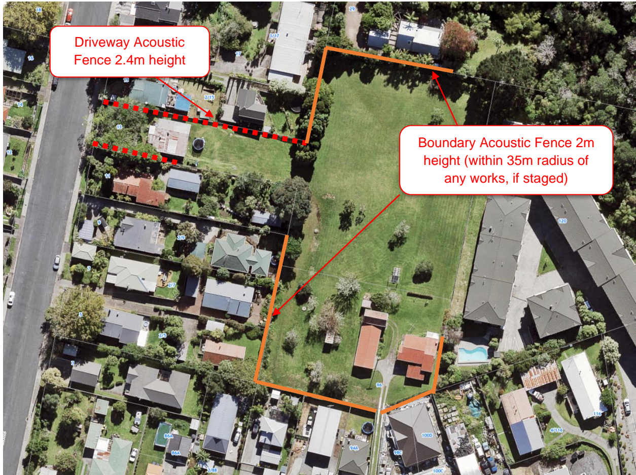
Figure 9 - Work Area boundary fencing - within 35m radius of area of works (if staged)
